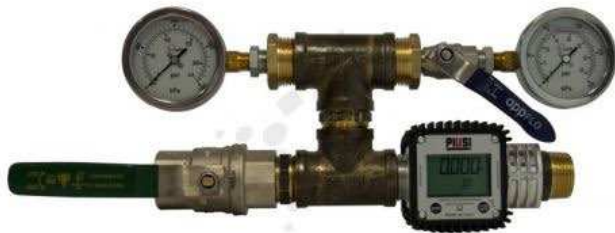
Pressure testing equipment
